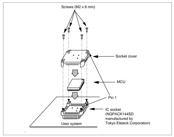
Figure 9 Installing MCU to User System
